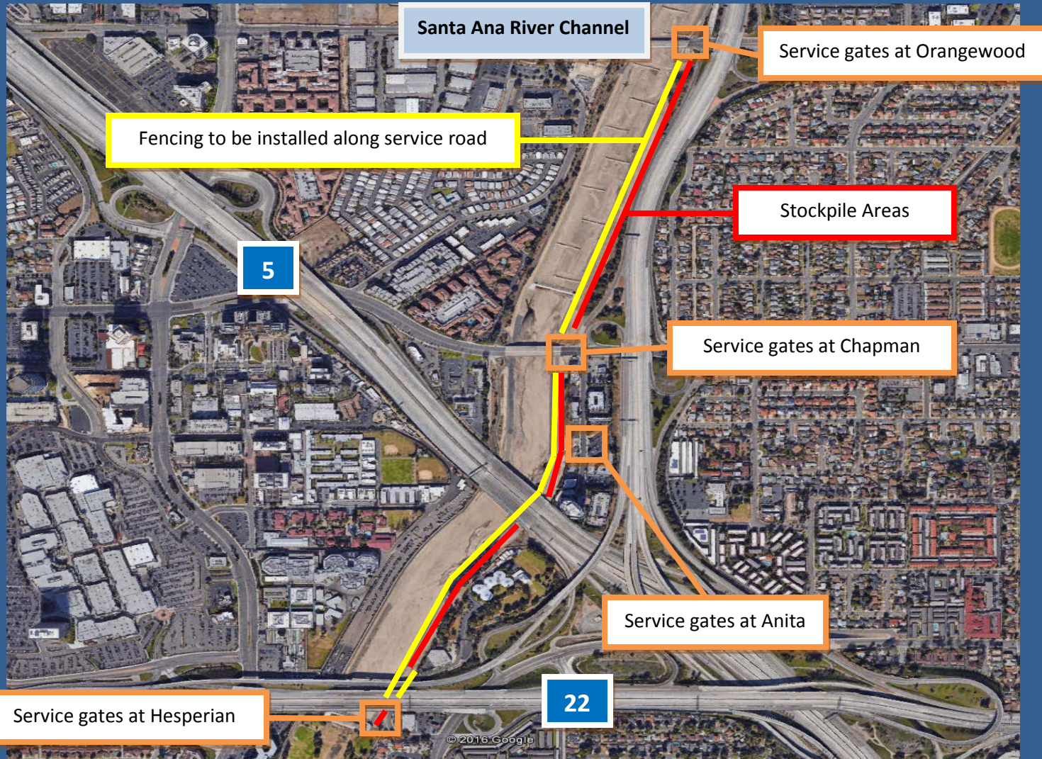
OC Public Works Stockpile Site and Fencing Project 2017
